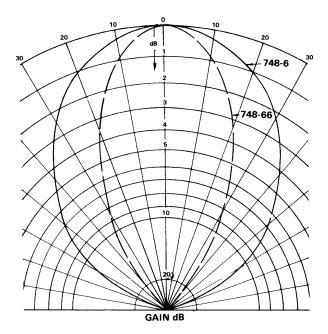
Gain: Model 748-6 = 15.2 dBi at 6 MHz, 16.2 at 30 MHz Model 748-66 = 18 dBi at 6 MHz, 19 dBi at 30 MHz 30 MHz
